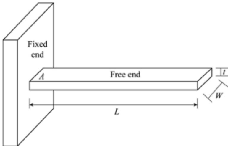
How do we calculate the deformation of a cantilever beam under known load?
